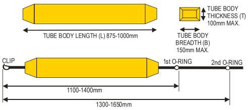
The distance from the extremity of the clip to the extremity of the first O-ring shall be a minimum of 1.10 m to a maximum of 1.40 m.
